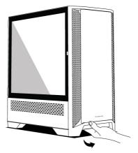
Open the front cover by pulling outwards with controlled force.
