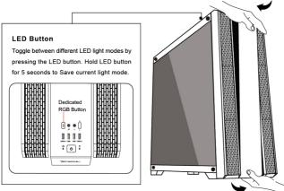
Open the top cover by pulling it upwards. \*Take caution when removing panels to prevent damaging I/O Connectors
