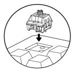
STEP 4: Inserting a new switch.
